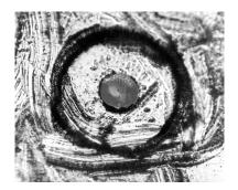
Figure 24 Damage from improper cleaning.
