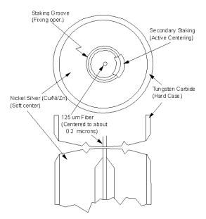
Figure 21 Cross-section of the Diamond HMS-10 connector.
