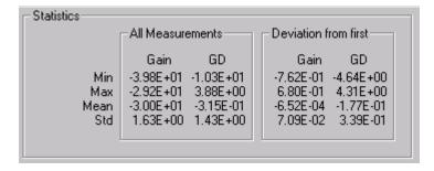
The statistics are calculated for Gain and Group Delay. The All Measurements block is calculated treating all wavelengths of all measurements equally. This is useful for measuring very flat and stable
