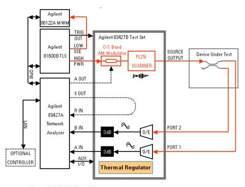
Figure 4 86038A Block Diagram
