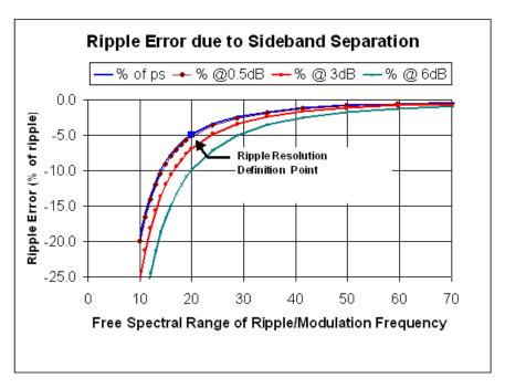
Figure 7 Ripple Error Due to Sideband Separation
