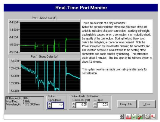
Figure 11 Example of a Dirty Connector
