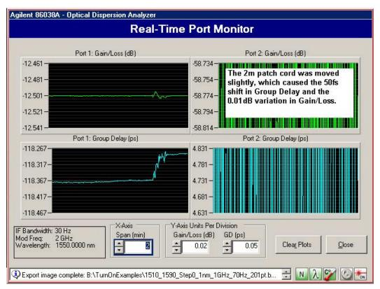
Figure 10 Example of Fiber Movement
