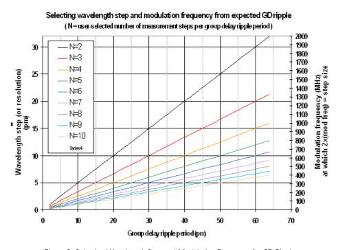
Figure 8 Selecting Wavelength Step and Modulation Frequency for GD Ripple
