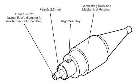
Figure 19 Basic components of a connector.
