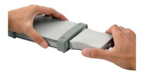
Figure 1. U2922A with U2751A used as a standalone device
