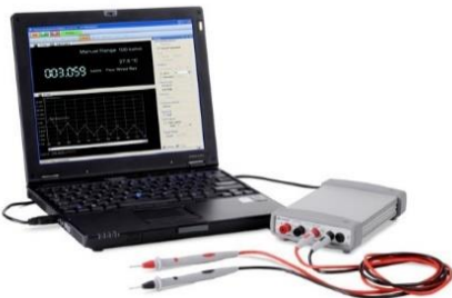
Figure 2. U2741A used as a standalone instrument
