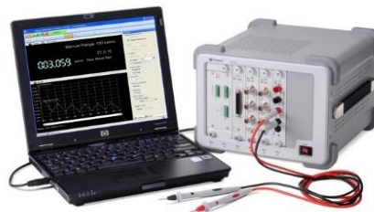
Figure 3. U2741A used as a modular instrument
