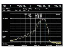
850 nm VCSEL Spectrum Measurement Example
